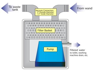
In a word, **Explanation:** The Auto Pump-Out connects inline with your vacuum hose. The 1,500 gallon per hour pump pulls waste water through the stainless steel filter and pushes it out the filtered water output valve. The Auto-Pump disposes almost all of the waste water before it enters the waste tank enabling you to work all day without stopping to drain your tank.
