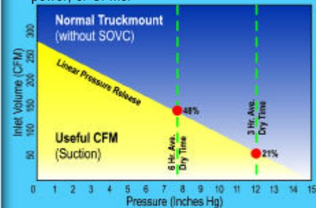
The SOVC kit replaces the manual relief valve with an electronically-controlled valve system that safely maximizes the suction power of your truckmount. As the chart below shows, SOVC delivers a massive power boost and cuts dry times dramatically.
